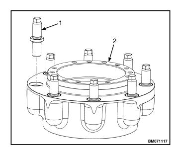
Figure 21. Wheel Studs Install for Lift Truck Models S4.0, 4.5, 5.5FT, S5.5FTS (S80, 100, 120FT; S80, 100FTBCS; S120FTS; S120FTPRS) (H004, J004)
