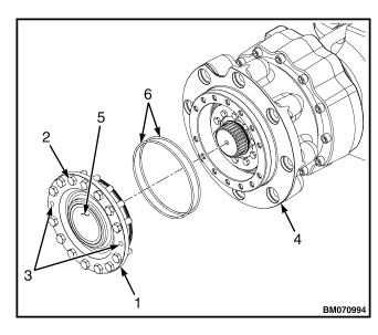
Figure 10. Wheel Hub Coupler for Lift Truck Models H4.0FT5/FT6; H4.5FTS5, H4.5FT6, H5.0-5.5FT (H80, 90, 100, 110, 120FT) (R005, S005, U005)
