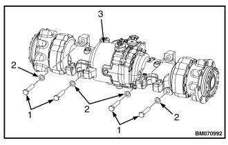
Figure 6. Drive Axle Mounting Capscrews
